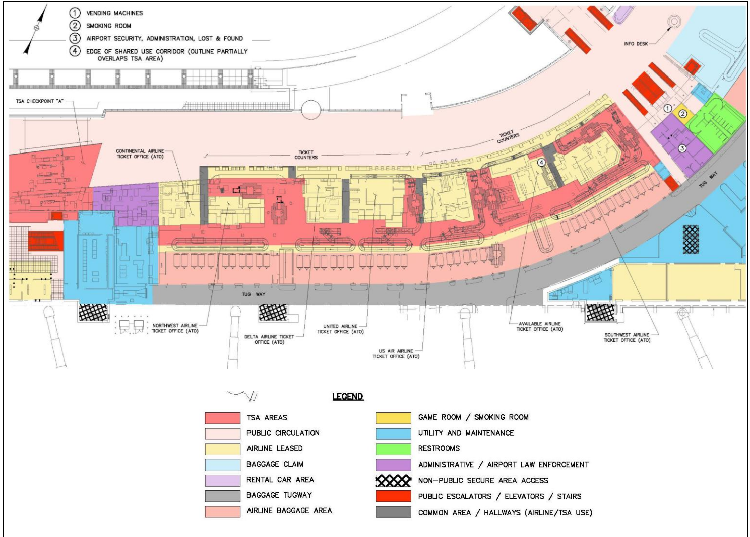
FIGURE 2-7 AIRPORT TERMINAL BUILDING, FIRST FLOOR DETAILS
